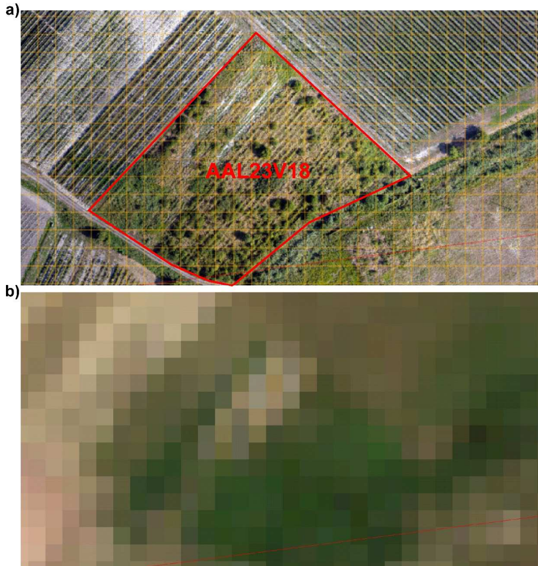
Figure 6: Differences between (a) detailed UAV-orthophotomosaic of the site PN8 – Dubová with the class AAL23V18 with 10 m pixel fishnet and (b) Sentinel-2A representation of the identical area.
